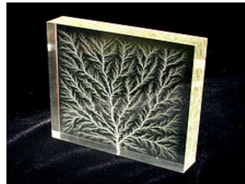
Fig.4. Dielectric breakdown within a solid insulator can permanently change its appearance and properties.
